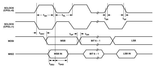
Figure 56. SPI Master Mode Timing (CPHA = 1)
